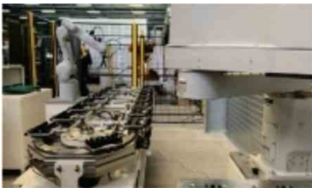
At its pilot plant, ProxinnoV has created a new robotic line for dismantling small household appliances and batteries - Photo :
