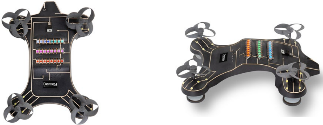
©DEMGY - Example of an additive manufacturing demonstrator with addition of selective metallization for electrical conductivity
